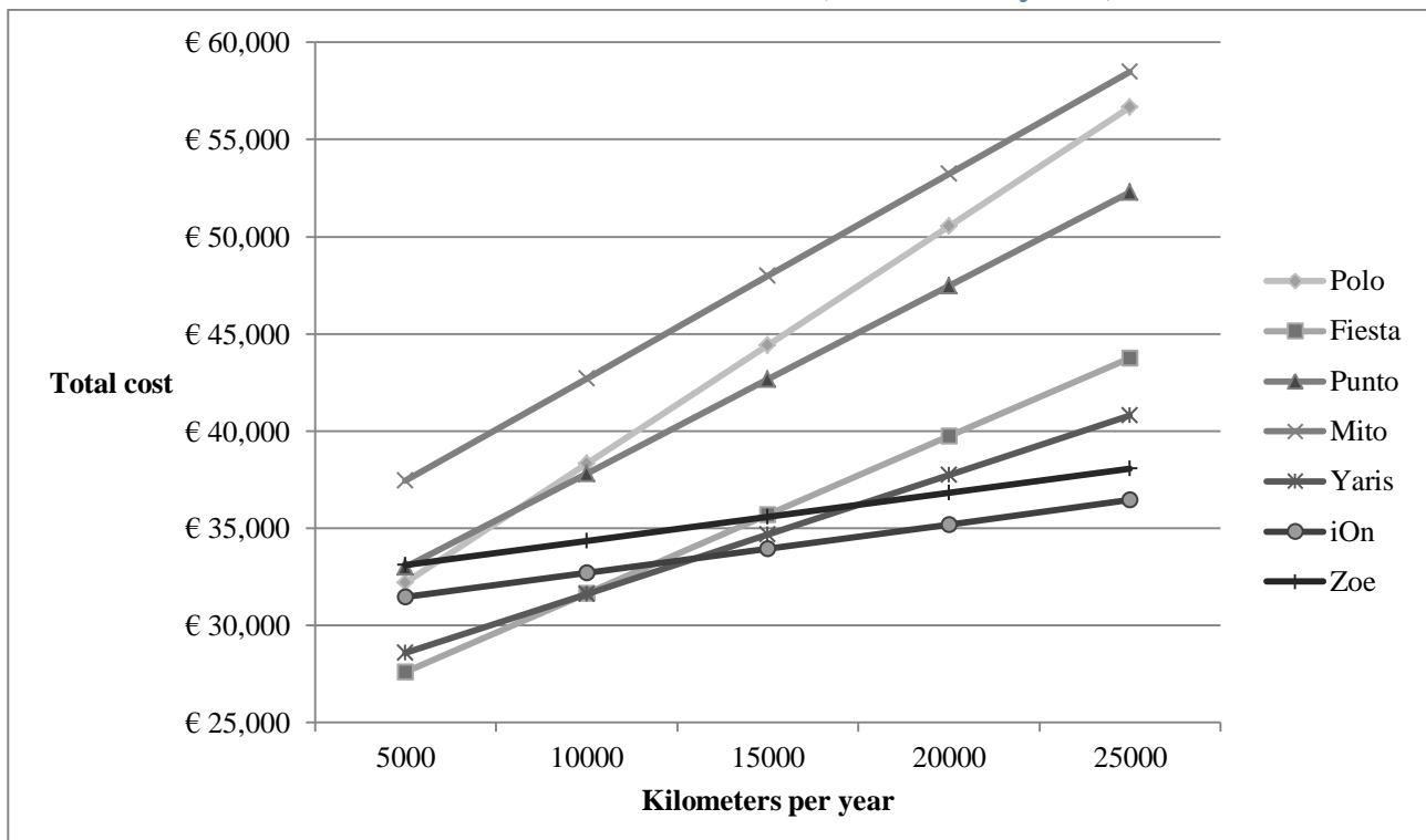
Figure 13- Total cost for different kilometers driven, given the Italian subsidies for less polluting cars in 2013 and 10 usage years
