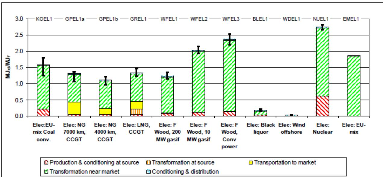
Figure 9 – Total energy balance for various electricity pathways. Source: \*Concawe, Eucar, JRC/IES (2007, p. 84)
