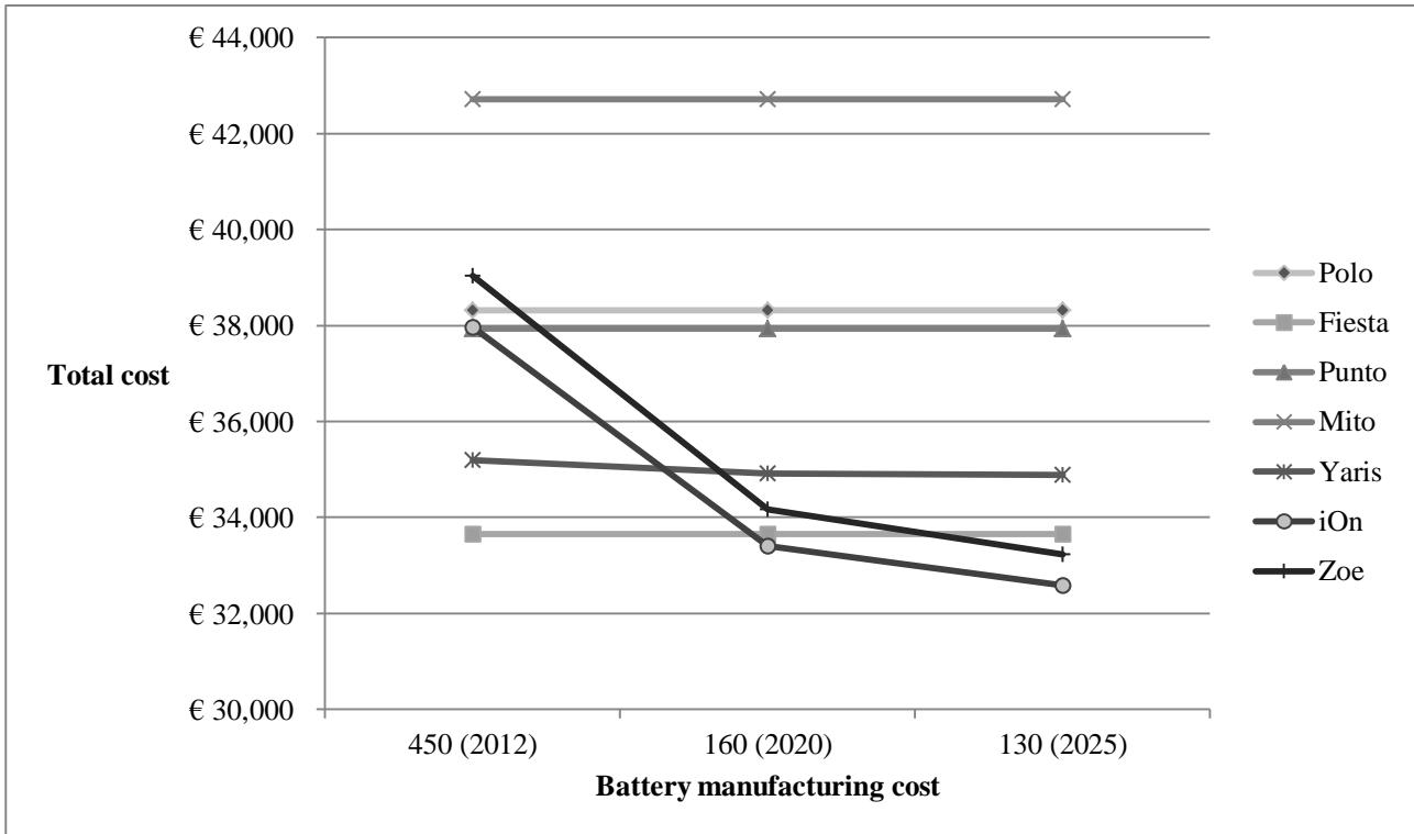
Figure 17 - Total cost with McKinsey battery manufacturing costs forecasts, given 10.000 kilometers driven per year and 10 usage years
