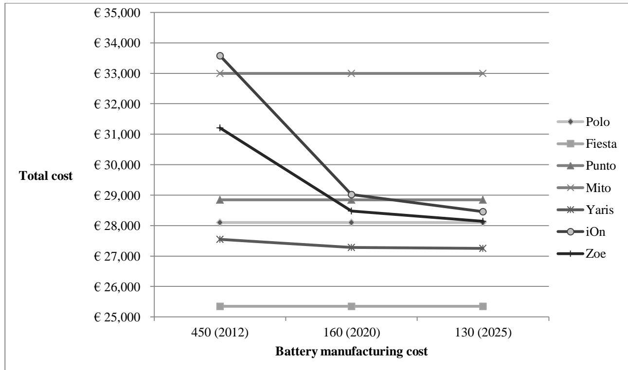
Figure 16 - Total cost with McKinsey battery manufacturing costs forecasts, given 10.000 kilometers driven per year and 5 usage years
