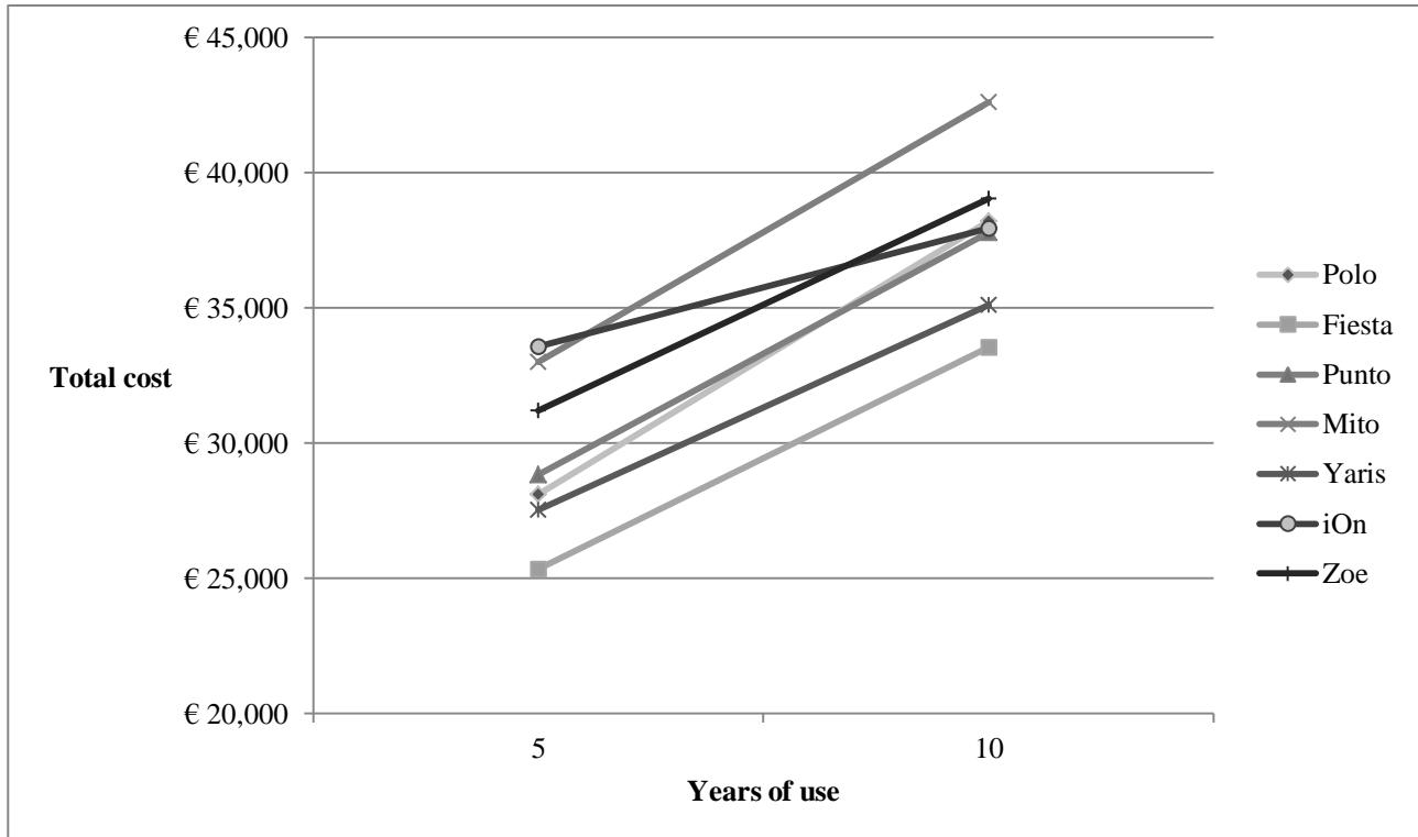
Figure 11 - Total cost for different usage years, given 10.000 km driven per year
