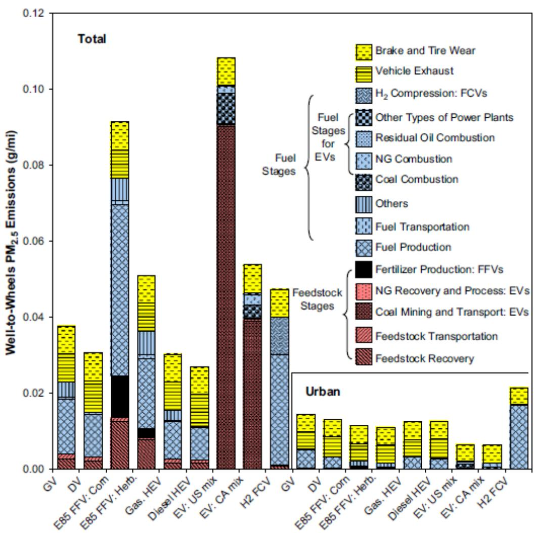
Figure 4 – WtW PM<sub>2.5</sub> emissions. Hou et al. (2009, p. 1802)
